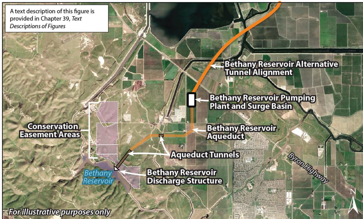
Figure 3-32. Bethany Reservoir Aqueduct Route with Tunnel Reaches
